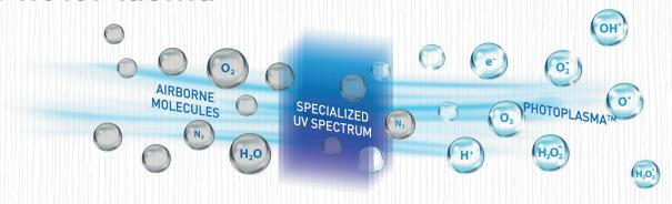
PhotoPlasma™ is generated by airborne molecules such as oxygen and water vapour under the exposure of the specialized UV spectrum. It includes reactive oxygen species, free radicals, electrons, etc., which actively capture various air contaminants, and rapidly destroy their structures through a chain of reactions. In this way the contaminants are decomposed and converted into harmless end-products like carbon dioxide and water.
